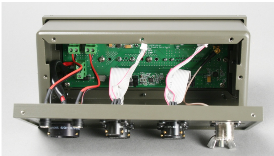
Cradle with rear open exposing the internal Cradle Interface PCB
